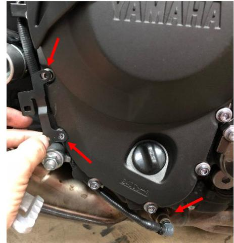
**Fig 1. O2 Sensor Location & Bracket Removal**
