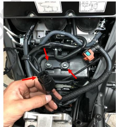
**Fig 2. Rerouting O2 Port & Charcoal Can**
